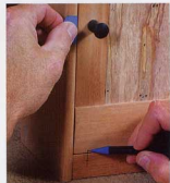
With the case assembled, transfer the mortise location. Use a piece of tape to pull the door flush with the outer edge of the case.
