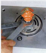
Above-the-table bit changes. Both ProLift models let you raise the router collet above the table, so bits can be changed from on top.
