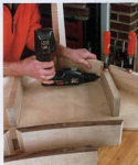
Install the drawer rails. Once the rails have been cut to length and aligned with the side rails using the template, secure them with screws.
