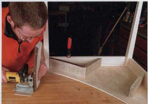
Biscuits join the apron to the drawer rails. The sharp angle at the end of each front rail demands care when using the biscuit joiner.
