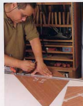
Cut triangles off the top. Use a straightedge and mat knife for quick, clean cuts.
