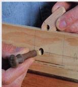
The knob should slide in with a little pressure. The spinner must swing freely and should be hidden when the latch is open.
