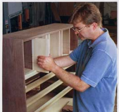
Begin with the vertical dividers. Once all of the joinery has been cut, the parts simply slide into place from the back of the case.
