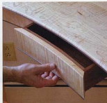
A place for your stuff. The drawer blends in with the front apron, making it nearly invisible. A fingerhold in the false front is easy to grab.
