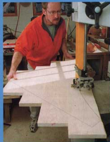
Rough-cut the tabletop after tracing the template. Minimize the waste of wood by stepping the glue-up to create a semi-triangular shape.
