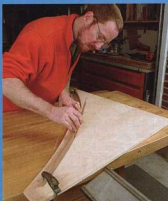
Draw the curve on the template. A thin wood batten and a piece of string yield a curve whose radius is adjustable. It's easy to transfer the curve to the template.
