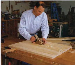
Use two points of pressure with wide stock. Multiple stops help keep wider stock from moving sideways during planing.
