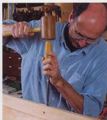
Chop out the mortise. Becksvort chisels out the mortise by hand.
