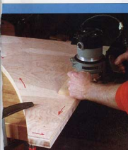
Flush-trim the edges. Using the template as a guide, flush-trim the edge of the tabletop. The arrows on the template indicate the routing direction to minimize tearout.
