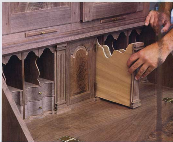
Installing a desk gallery, p. 66
