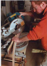
Trim the front apron on a chopsaw. The false drawer front is cut at an angle to preserve the seamless appearance of the apron.
