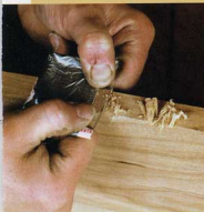
The planing cut. For a smooth, burnished finish, hold the glass as you would a low-angle plane blade.
