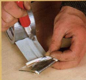
For safety, wrap the three unused sides of the scraper with electrical cable insulation. Secure it with duct tape.
