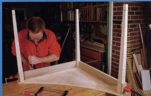
Assemble the rear of the table. After the legs and the side aprons have been cut, glue them together using the template as a guide to squaring them up.
