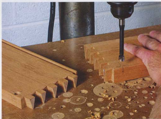
Drill mortises before gluing up the case. One set of magnets is recessed into mortises drilled into both the case top and bottom.
