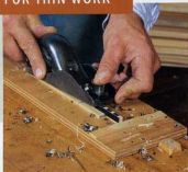
Planing thin, straight stock. This jig is simply a piece of plywood with thin, perpendicular fences. Butt the jig against a benchdog to hold it in place.
