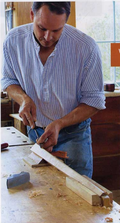
Planing thin, straight stock. This jig is simply a piece of plywood with thin, perpendicular fences. Butt the jig against a benchdog to hold it in place.
